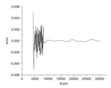
Fig. 4. The relative error between the object spectrum and the numerical inversion results from the simulated attenuation data without noise.
