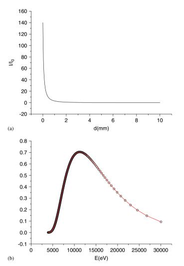
Fig. 3. (a) The simulated attenuation curve without noise; (b) the solid line is the object distribution. The circles are the numerical inversion results from the simulated attenuation data without noise.
