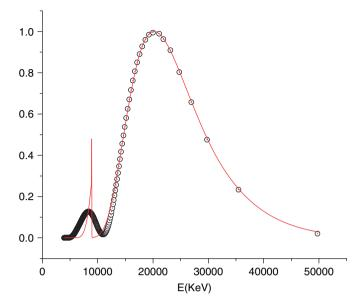
Fig. 8. The solid line is the theoretical result of the white light absorbed by Cu. The circles are the numerical inversion results. The position of Cu absorption peak has an error level of 6%.
