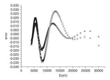
Fig. 6. The triangles are the error between the object distribution and the numerical inversion results from the simulated attenuation data with Gaussian random white-noise level in [-0.1, 0.1] and the circles are those in [-1, 1].
