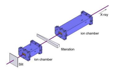
Fig. 1. Outline of the experimental setup. The slit was used to limit the incident X-ray to  $0.1 \, \text{mm}$   $(H) \times 1 \, \text{mm}$  (V).
