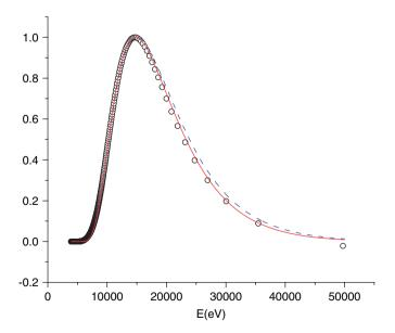
Fig. 7. The circles are the numerical inversion results from experiment data. The dash line is the theoretical distribution of the center of the light. The solid line represents the theoretical distribution after considering the beamline direction is offset from source central direction by 16.7 mrad.
